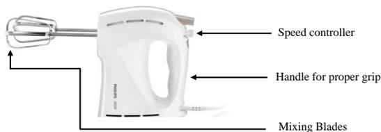
Fig 3.3.1. Hand held Foam generator for generating foam.
