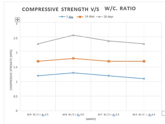
Figure 4.5: Comparison of Compressive Strength of samples with density 800 kg/m<sup>3</sup> but different water cement ratio.
