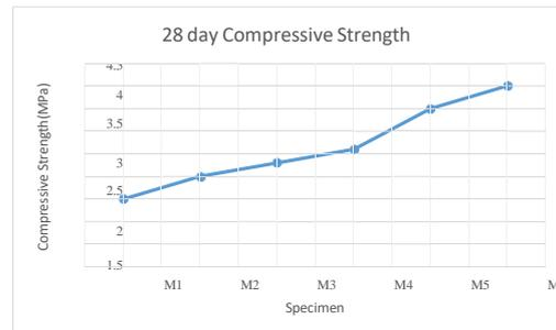
Figure 4.3: 28 day compressive strength of specimen (Trial mix set -1)
