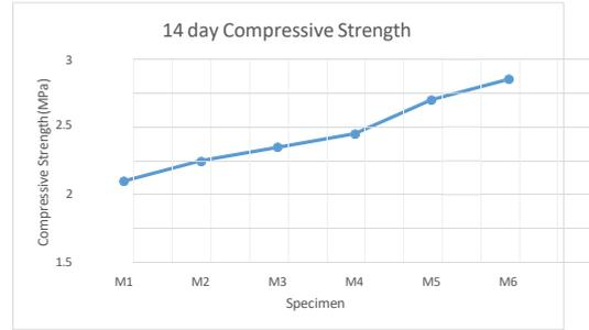
Figure 4.2: 14 day compressive strength of specimen (Trial mix set -1)
